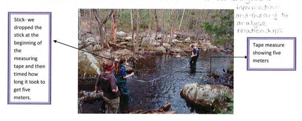
The test above was used for measuring the speed of flow. This could have been done more accurately if we measured the width of the site and stood right in the middle of it. Thus, ensuring each time we were measuring the flow from the middle of the river; or even easier and more accurately using a flow meter.
